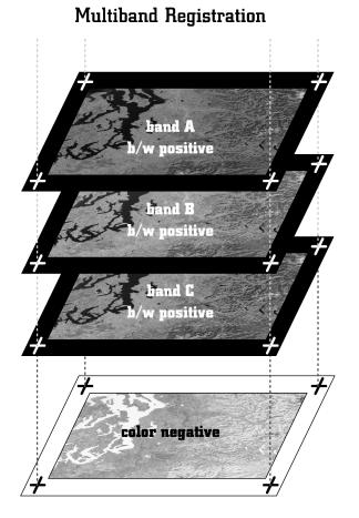
Figure 3. Multiband registration. The crosshairs in each corner of the film separations occupy the same pixel address among all three black-and-white positive records. Their accurage registration assures a controlled composite in the first generation color negative.
