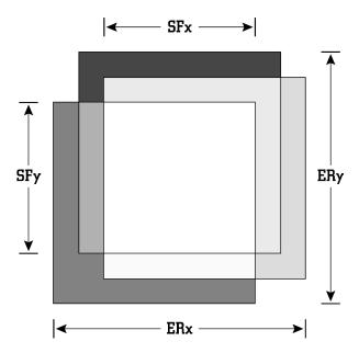
Figure 5. A white pixel with SF .64 / ER 120%. When registration is perfect, the signature factor will have a value of 1.00 and the effective spatial resolution will equal the design specifications of the imaging system. Gathering accurate information is the objective of remote sensing and image analysts must know that the color signatures which form the image are valid expressions of energy detected by the sensors.
