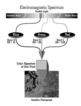
Figure 1. Color signature derivation. Color signatures can be validated when their radiometric integrity is preserved during the digital-to-analog conversion. The DNs assigned to the levels of detected energy must govern the color composition of individual pixels within the photographic hardcopy.
